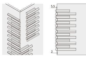
An external corner can be tiled with combinations of External Corner Starter Units and their vertically flipped Units (brick joint). Allow a joint width of 2 mm between the back faces of each unit and side faces of the combined units.
